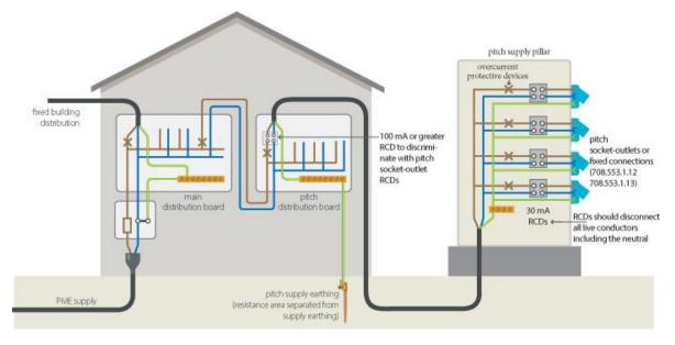
Alternatively, the separation of the earthing can be made at the caravan pitch supply points. In this instance, earth electrodes will be required at these points. See the below Figure 7.2 of IET Guidance Note 7 for detailed information.
